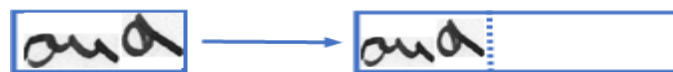
Fig. 4: Left: a picture from the dataset with an arbitrary size. it's scaled to suit the target image of size 128×32, the empty part of the target image is crammed with white color.
