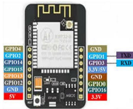
Figure 2: ESP32 CAM WiFi module
