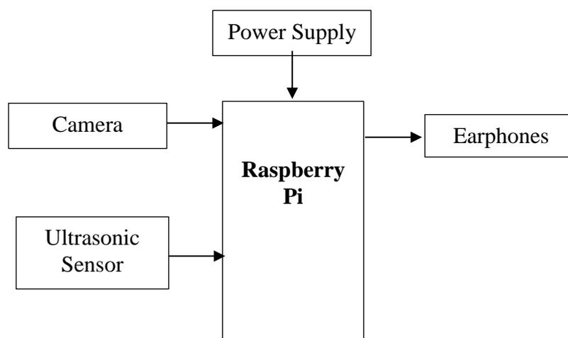
In this project we are using ultrasonic sensor for the people detection. When it detects the person then the image will be taken and is searched in the predefined data base. If the image matches, then the person’s name will be given as voice through earphone otherwise it will say unknown person.
