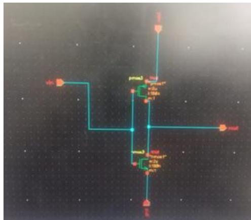
Fig 2:CMOS Inverter in schematic editor
