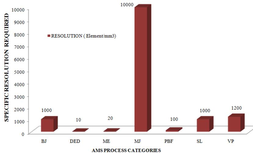
**Figure 5:** Specific resolution required in the additive manufacturing strategy process categories
