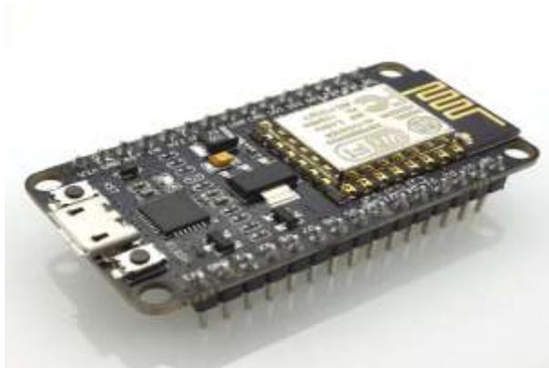
The ESP8266 wi-fi module is a self-contained soc with integrated TCP/IP protocol stack that can give any microcontroller access to your Wi-Fi network. The ESP8266 is capable of either hosting an application or offloading Wi-Fi networking from another application processor.
