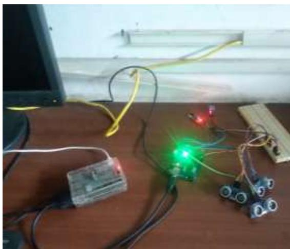
Figure3.1: Multiple Sensors connected with Arduino sensors
