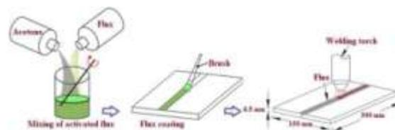
**Fig: 2. A-TIG welding process.**
