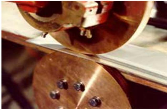
Fig. 4 RSEW producing continuous joint
