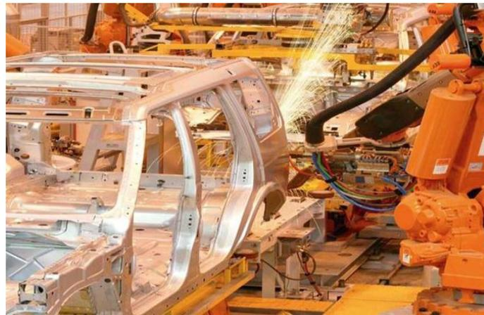
Fig. 2 Industrial robots welding car body (Source: Rexroth- Bosh group) [4]
