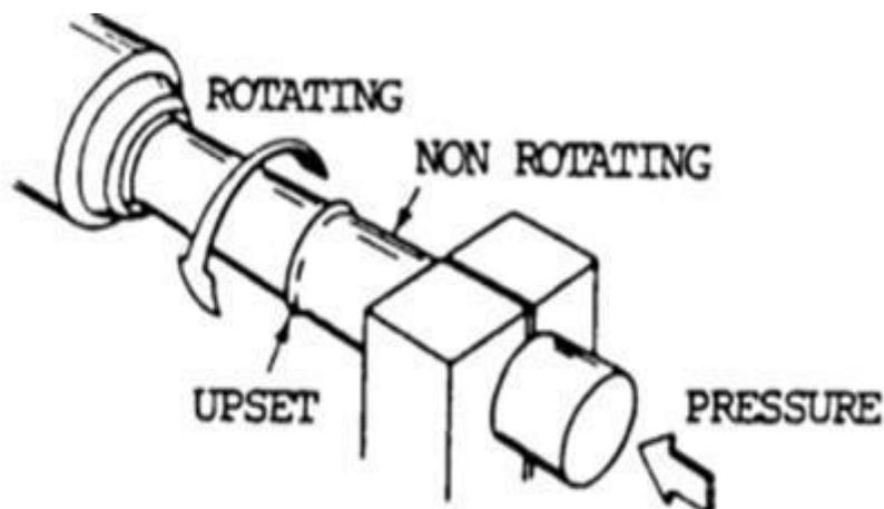
Fig. 5 Shafts joined by friction welding process
