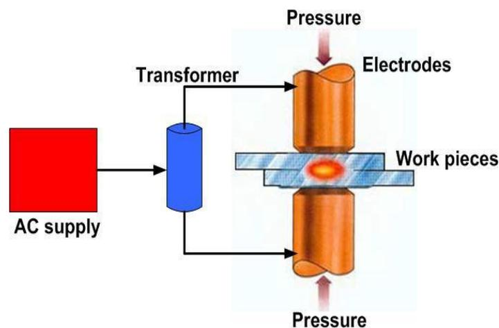
**Fig. 1 Resistance spot welding**
